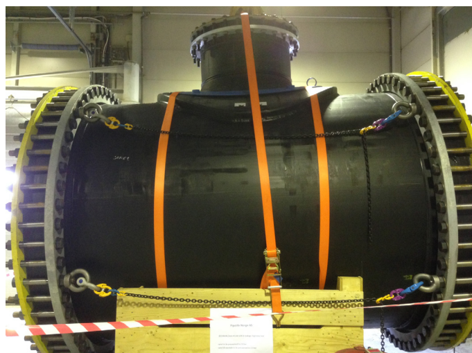
Full scale pressure test of OD1000 saddle on OD2500 pipe to 2 bar
