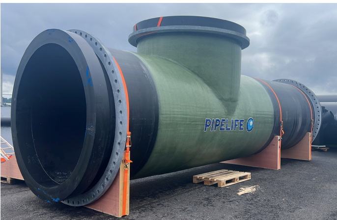
OD2500 mm fabricated tee with GRP reinforcing wrap.
